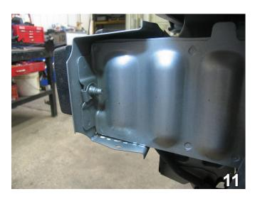
11. Using the reciprocating saw, cut the frame rail webbing flush with the bottom of the frame and the back of the metal bumper. Do this to both sides of the vehicle.
