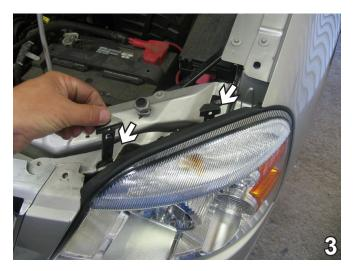
Pull up on two plates just behind headlight assembly to remove them. Pull headlight assembly forward, disconnect electrical and remove assembly. Do this to both sides of the vehicle. Set plates and headlight assemblies aside to be reinstalled later.
