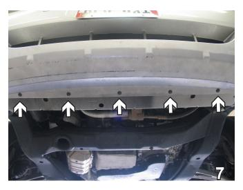
Remove nine Phillips screws, two each side and five in the center underneath the fascia. Pull forward on fascia to remove. Set screws and fascia aside carefully to be reinstalled later.
