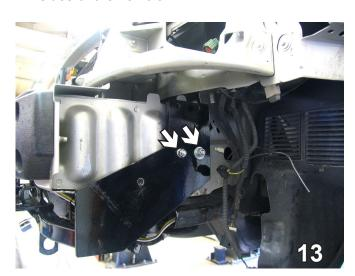
13. Align middle holes of baseplate with existing holes of frame. Insert two 3/8-16 bolt plates through the hole on side of frame rail and align with the two existing holes in the frame. Install 3/8" flat washer, 3/8" lock washer and 3/8-16 hex nut and tighten to bolt plates. Do this to both sides of the vehicle.
