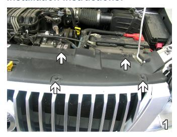
Remove four pushpins from the top of the radiator cover. Do this to both sides of the vehicle. Remove radiator cover. Set pushpins and radiator cover aside to be reinstalled later.
