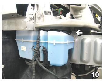
10. On the passenger's side, disconnect tubes and electrical connections from the washer reservoir and plug the reservoir. Using an 8mm socket, remove the metric bolt from the reservoir bracket. Set bolt and reservoir aside to be reinstalled later.
