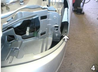
Using the 8mm socket, remove one metric bolt from the top corner of fascia. Do this to both sides of the vehicle. Set bolts aside to be reinstalled later.
