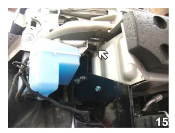
15. On passenger's side upper frame webbing, forward of the baseplate, drill out the front washer reservoir hole with the 9/32" drill bit (see white arrow). Reinstall the washer reservoir bolts. Insert the 1/4-20 x 2 1/2" hex bolt into 1/4" flat washer, forward washer reservoir hole, 1/4" flat washer, 1 1/2" pipe, 1/4" flat washer, drilled hole, 1/4" flat washer and tighten to 1/4" lock washer and hex nut.
