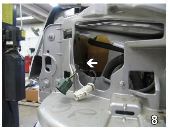
Behind the passenger's side headlight assembly, use the 8mm socket to remove one metric bolt from the inside wall of the fender well. Set bolt aside to be reinstalled later.
