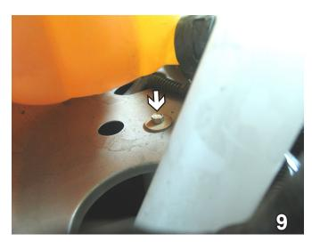
9. On the bottom of the passenger's side fenderwell, use the 8mm socket to remove one metric bolt. Set bolt aside to be reinstalled later.
