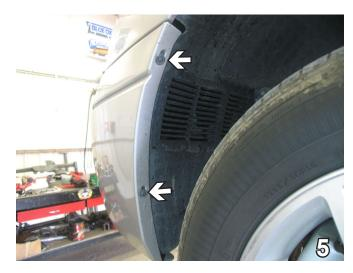
Just inside wheel well, on edge of fascia, remove two Phillips screws. Do this to both sides of the vehicle. Set screws aside to be reinstalled later.
