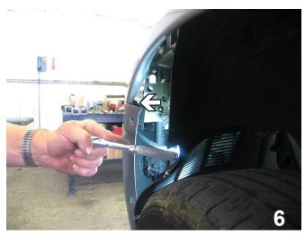
Push wheelwell cover aside and remove one metric bolt using the 10mm socket. Do this to both sides of the vehicle. Set bolts aside to be reinstalled later.
