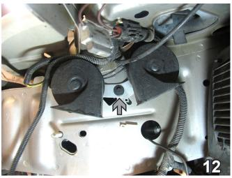
12. On the driver's side, disconnect electrical and use the 8mm socket to remove one metric bolt from the horn bracket. Remove horns. Set bolt and horns aside to be reinstalled later.
