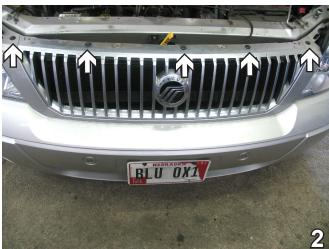
Remove five pushpins from the top of the grille. Set pushpins aside to be reinstalled later.
