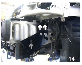
14. Using the baseplate as a template, drill three remaining holes into frame using the 13/32" drill bit. In the upper two holes (see white arrows), insert 3/8-16 x 2" hex bolts and tighten to the 3/8" lock washers and 3/8-16 hex nuts. In the lower hole (see grey arrow), insert a 3/8-16 x 2" hex bolt and tighten to the 1/2" pipe, 3/8-16 hex nut and 1/4-20 x 2 1/2" hex washer. Do this to both sides of the vehicle.
